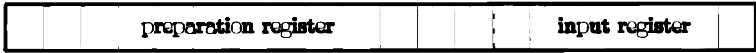
Fig. 1. The input port consisting of a preparation register and an input register.
